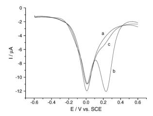
Fig. 4. Square-wave voltammograms of AgCl@PANI/GC electrode. Curve (a): pH 7.0 phosphate buffer; Curve (b): (a) +0.1 mM dopamine; Curve (c): (a) +1 mM ascorbic acid.
