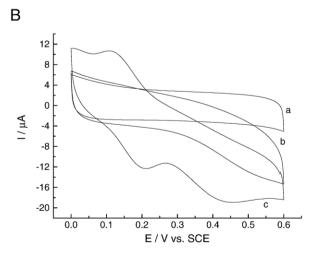
Fig. 5. Molecular structures of PVP (a), dopamine (b), ascorbic acid (c) and intramolecular hydrogen bonding of ascorbic acid (d) (A).Cyclic voltammograms of PVP modified GC electrode. Curve (a): pH 7.0 phosphate buffer (0.1 M); Curve (b): (a) +1 mM ascorbic acid; Curve (c): (a) +1 mM dopamine (Scan rate:  $0.1 \text{ V s}^{-1}$ ) (B).
