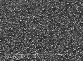
Fig. 1. SEM images of AgCl@PANI nanocomposite (up) and Nafion coated AgCl@PANI nanocomposite films (down) on silicon wafers.
