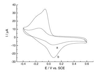
Fig. 6. Cyclic voltammograms of AgCl@PANI/GC electrode (a) and Nafion–AgCl@PANI/GC electrode (b) in pH 7.0 phosphate buffer (0.1 M). Scan rate:  $0.1~{\rm V~s}^{-1}$ .
