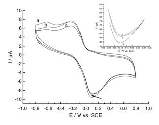
Fig. 3. Cyclic voltammograms of AgCl@PANI/GC electrode. Curve (a): pH 7.0 phosphate buffer (0.1 M); Curve (b): (a) +1 mM dopamine; Curve (c): (a) +1 mM ascorbic acid (Scan rate: 0.1 V s $^{-1}$ ). The insert shows the enlarged view of the region indicated by the arrow.
